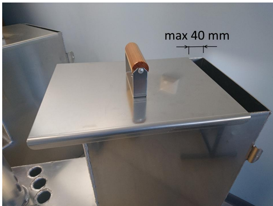
Image 4. Maximum lid opening during heater use
