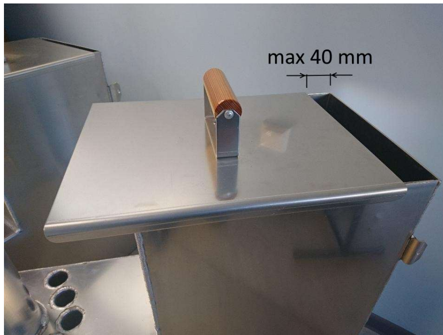
Image 4. Maximum lid opening during heater use
